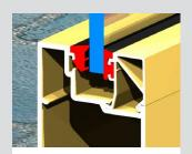
Series 51 doors are screwed together with #10 stainless steel screws and heavy duty extruded aluminium backing plates.
